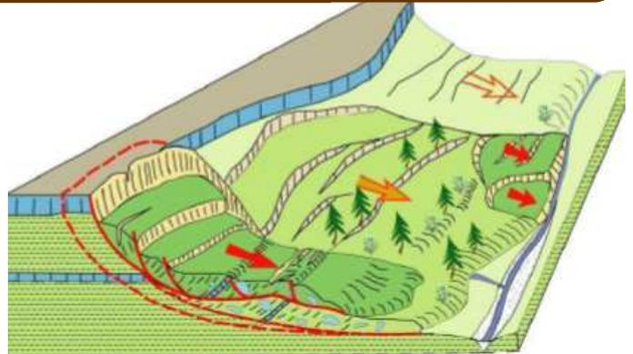
CONCEPTUAL DIAGRAM OF LANDSLIDE PHENOMENON
