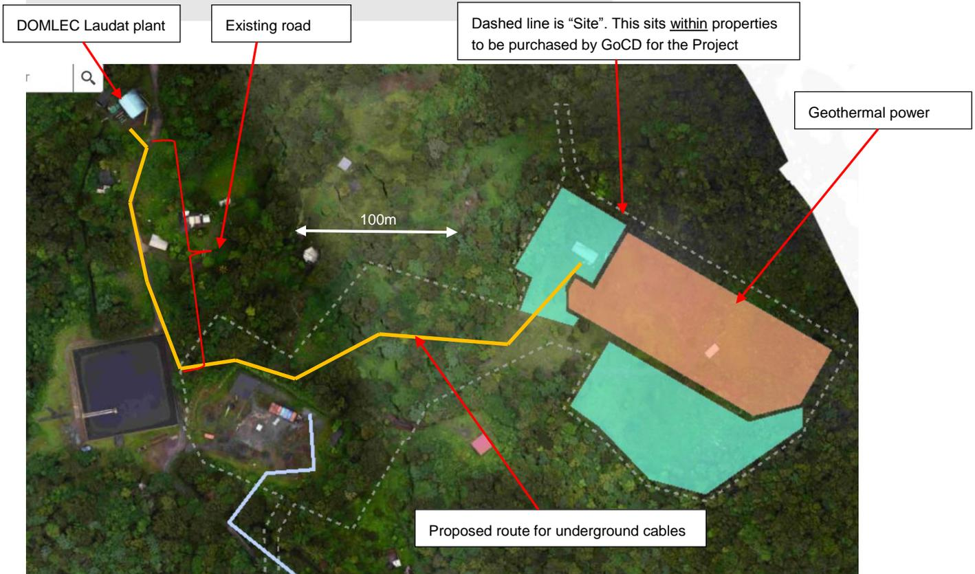
Figure 4-13 : Proposed connection with DOMLEC Grid
