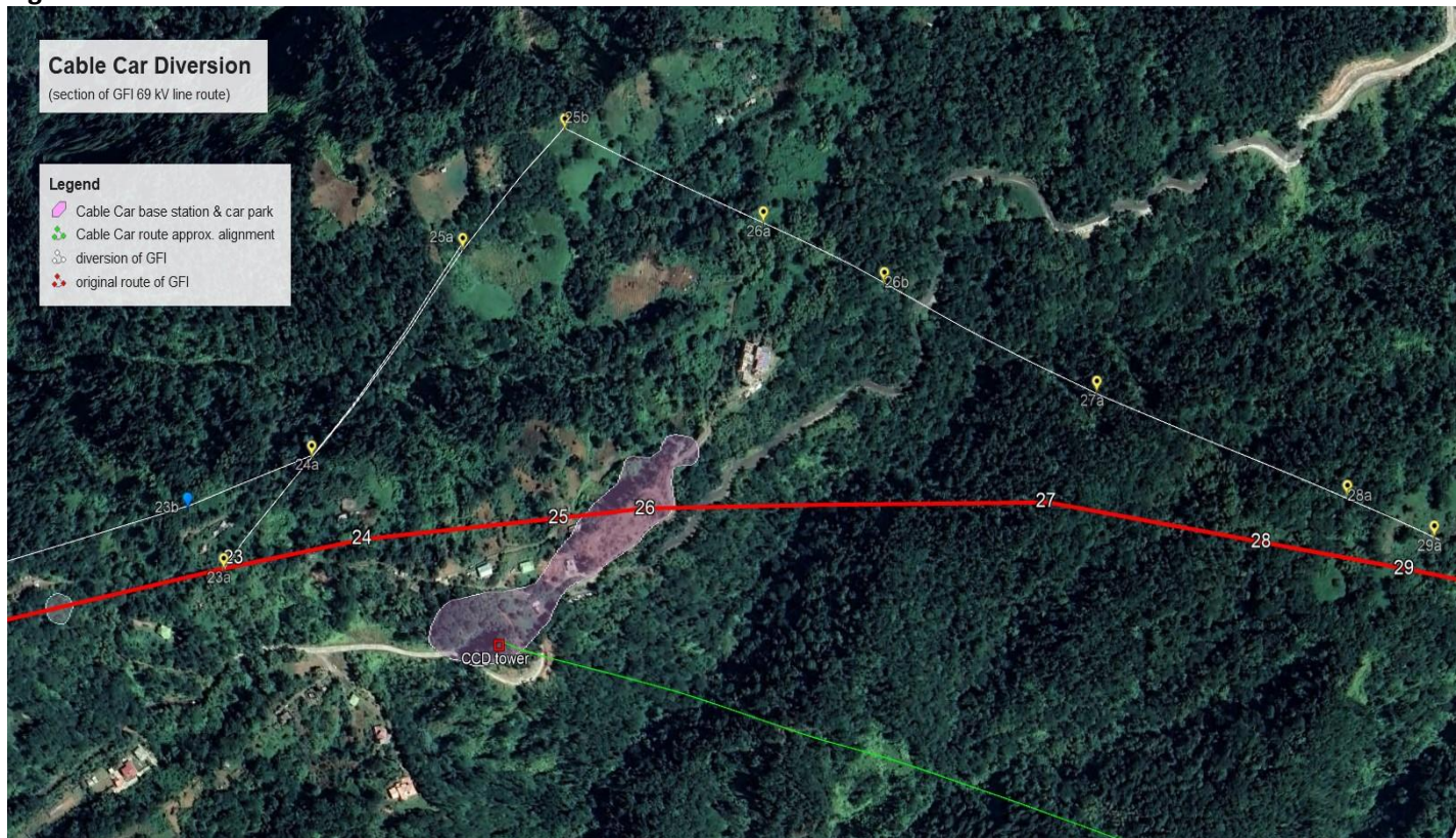
Figure 6. Diversion Due to Cable Car Installation
